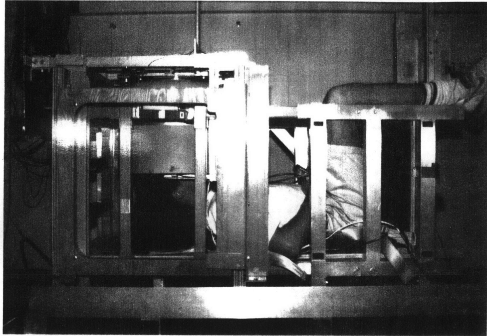
Figure 3.7. Rotating dome and magnetic field coils in erect and supine orientations. [a.] In the erect position, the coil system rests on two tables, and the subject stands within the coil frame. [b.] For the supine runs, the coils are supported by the chair designed for the MIT linear acceleration sled, and the subject lies in the chair.
