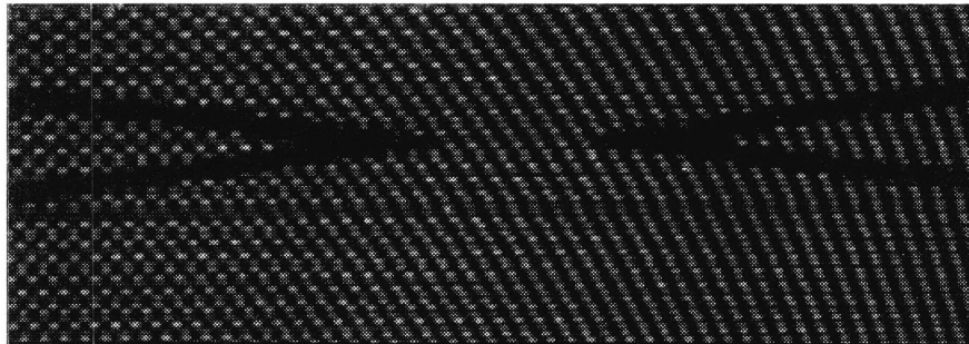
Figure 7-1: Bad 'Seam' on a Zone Plate
