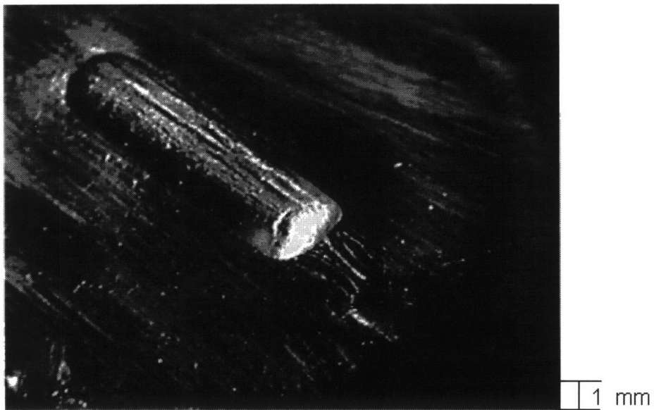
Multiple cracking at the final stage of the first loading cycle (C1).
