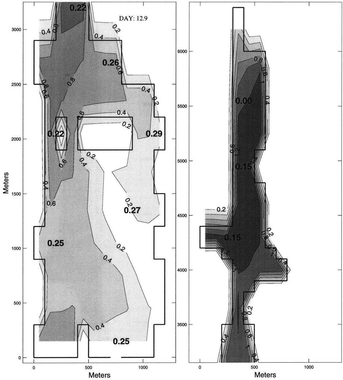
Figure 6-13: Simulated contours vs. ASA observations: December 28, 1986 Contours are simulated dye study. Values in bold are ASA (1987) observations
