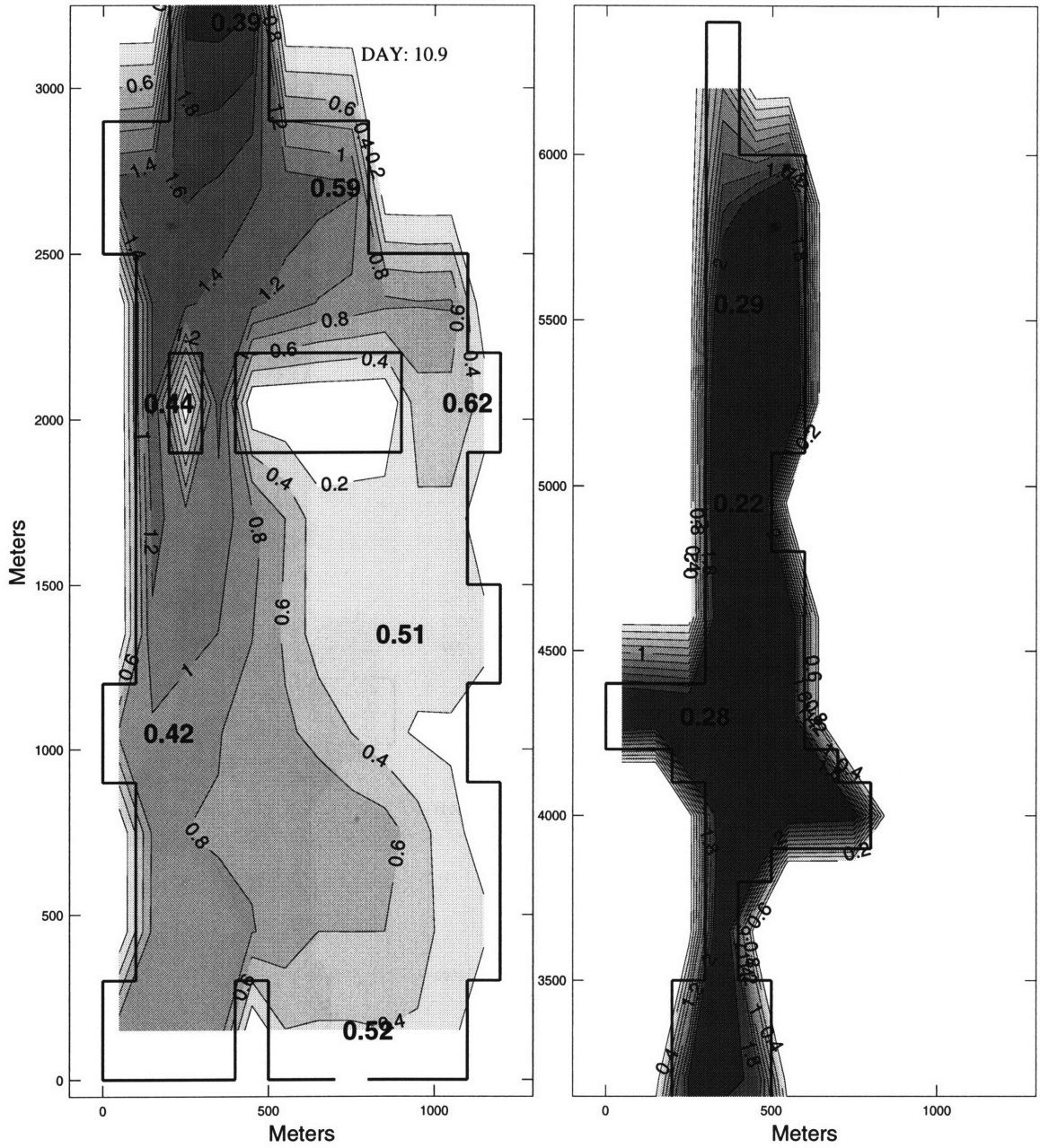
Figure 6-11: Simulated contours vs. ASA observations: December 26, 1986 Contours are simulated dye study. Values in bold are ASA (1987) observations
