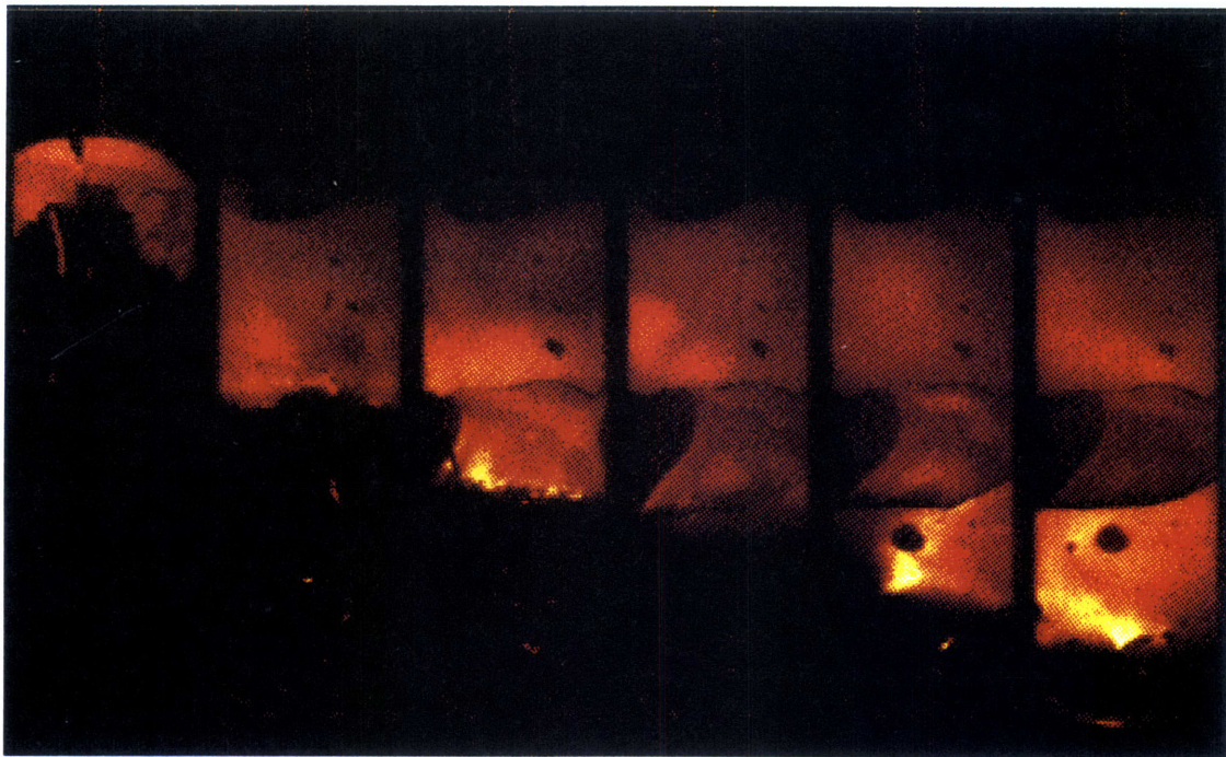
Fig. 5.6. False-color images of combustion front propagation and bubble formation at 320 ms time steps in Sample W10, N_{Ni} = 0.60 . Note the areas of changing intensity and hot spots. (Viewing window width \approx 1.25 cm.)
