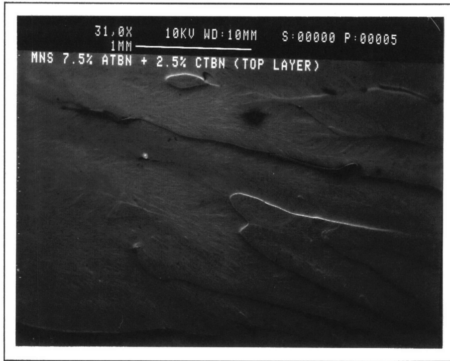
Figure 4.59- Plastic flow on the fracture surface of a sample taken from the top region of an MNS casting containing 7.5% ATBN and 2.5% CTBN.
