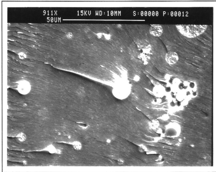
Figure 4.125- Well-adhered glass spheres on the fracture surface of an MNS compact tension specimen containing 12% ATBN and 5% hollow glass spheres reacted with an epoxy coupling agent.
