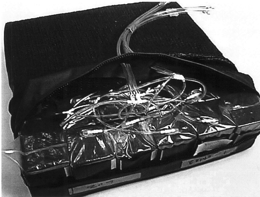
Figure 8: Active cushion, cover retracted showing tubing.
