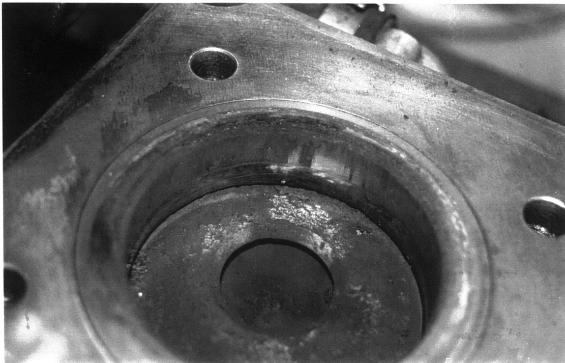
Figure 3.6 Deposits on piston and cylinder liner after 14 hours of pyrolysis oil operation.
