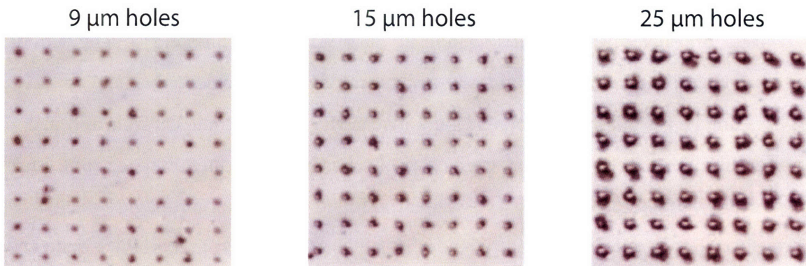
Figure 8-3: Close-up images of photonic crystals machined in 50 micron thick LN.
