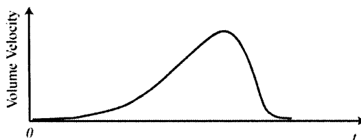
Figure 2-13. Schematic view of a glottal volume-velocity waveform, adapted from [54].
