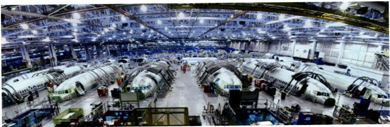
Figure 5 - Fuselage 737 Final Integration Assembly Area
