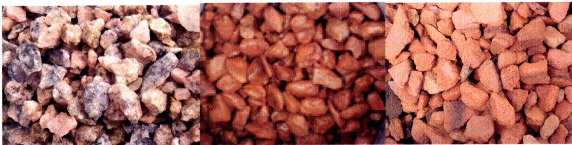
Figure 52 Pilot HRF media: granite gravel (G) left, local gravel (D) center, broken pottery (P) right
