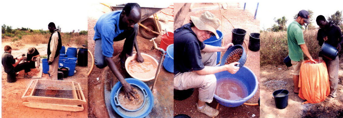
Figure 53 Breaking and sieving pottery (left), Baba cleaning pottery with sieves (center-left), Kim Weaver (Peace Corps) cleaning pottery (center-right), Carl Allen (Peace Corps) pre-filtering dugout water with bed sheet to remove copepods before using the water to clean local gravel (right)
