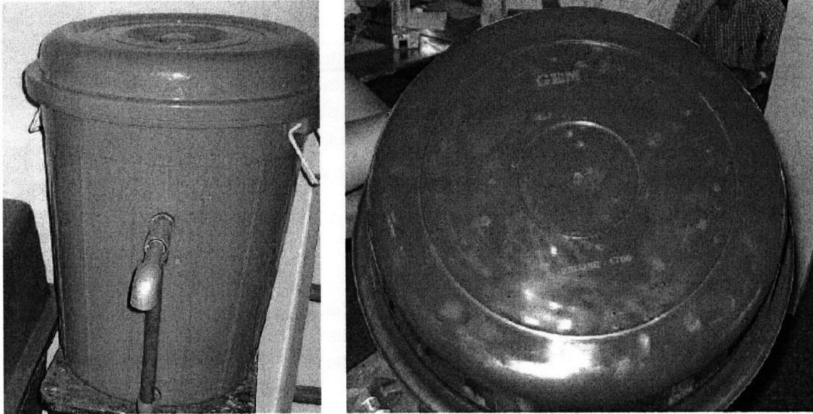
Figure 5-3 Picture of a LPD BSF and Diffuser Basin
