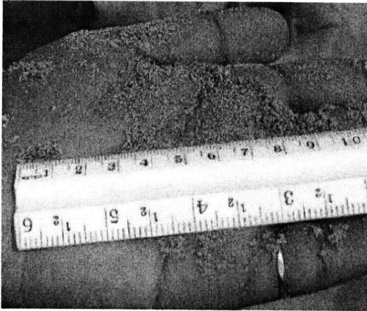
Ideal fine sand - correct size, no large particles or visual contamination
