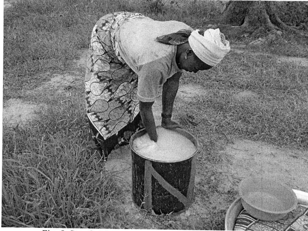
Fig. 5. Step 2: Manual coagulation with one alum ball
