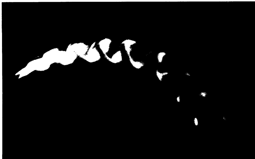
Fig. 13. Von Kármán trail generated by cylinder moving in a circular arc.
