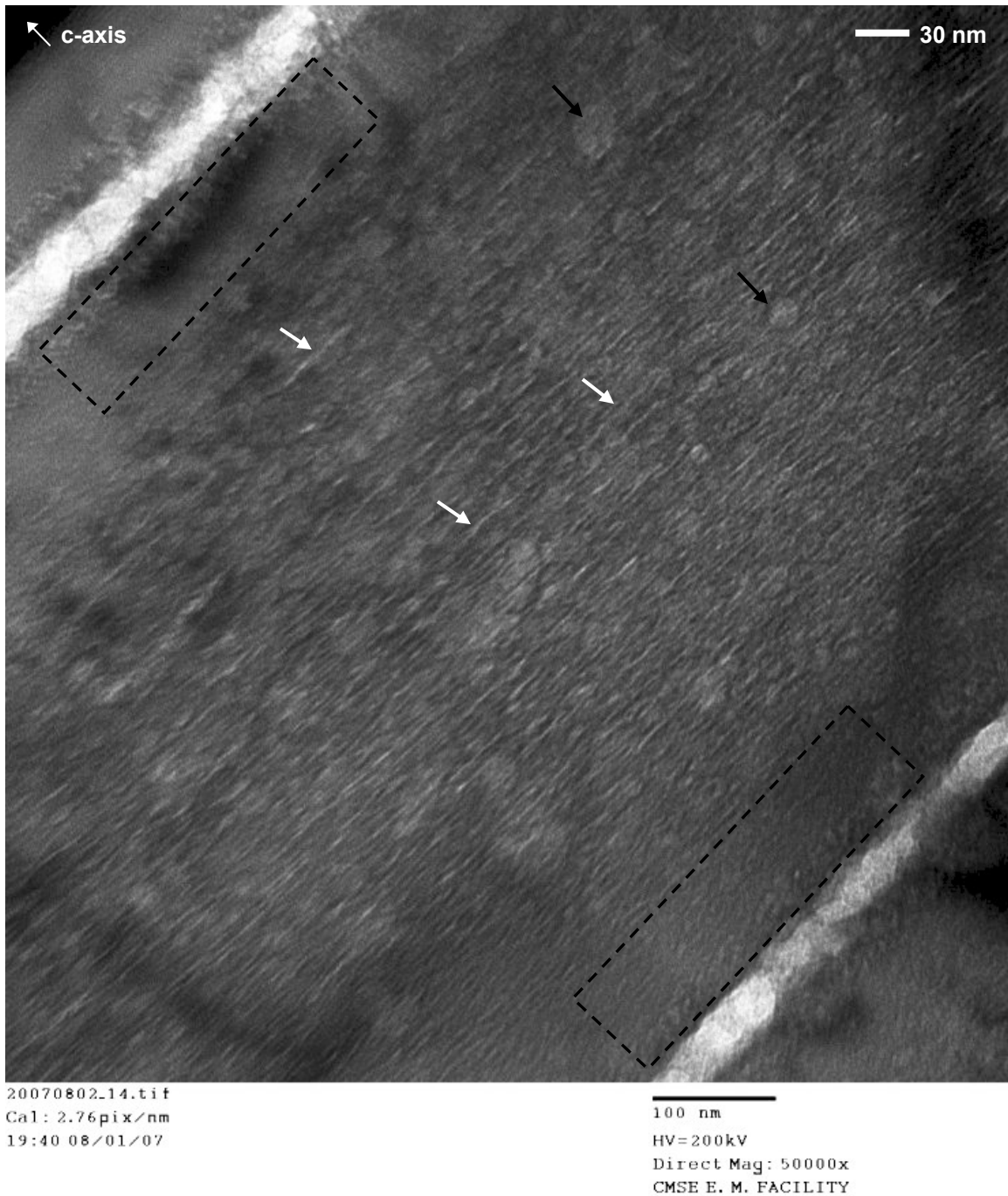
Fig. 3.23 TEM image of a FIB-prepared section from the cross-section of a nacreous tablet from fresh H. rufescens . Image by D. Alcazar.
