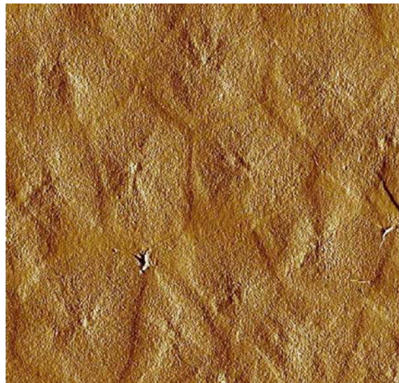
Fig. 3.9. Contact mode deflection atomic force microscopy (AFM) image of top down view of inner laminate columnar nacre of T. niloticus nacreous layer fractured in uniaxial compression 30 \mu\text{m} scan.
