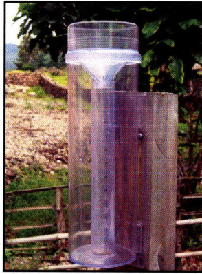
Figure 3-13: Rain gauge at trackers' house
