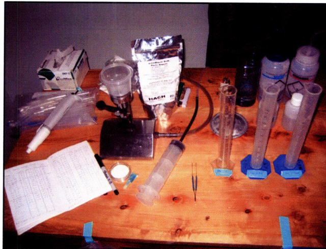
Figure 3-6: Membrane Filtration Equipment
