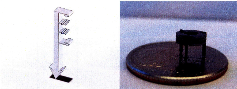
Figure 3-10 A modified three-dimensional device (left: schematic view of a modified clamp, right: an assembled device on a quarter).
