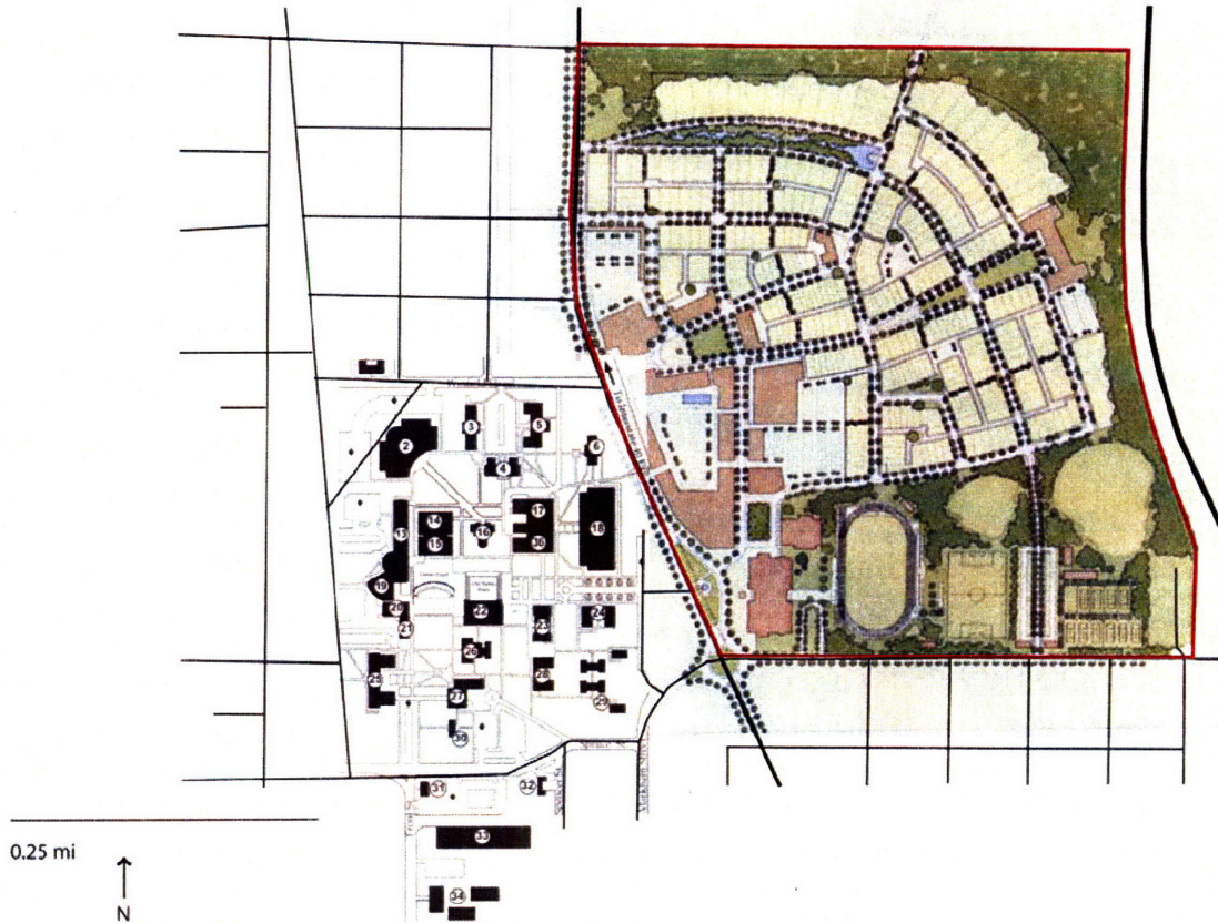
Figure 4.3: The plan of The Village at Hendrix (color) inserted into a plan of the Hendrix College campus and the existing street grid of Conway clearly reveals that the new village is about the same size as the campus. The campus and the village have a nice symmetrical relationship with a clearly defined edge at Harkrider Street. Both the campus and the village connect to the street grid, yet they remain separate from it with internal networks of streets and quadrangles. (Diagram by the author, with campus map and project site plan)
