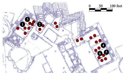
FIGURE 5-19—Experimental Zigbee testbed layout: there are 31 nodes in total, spread over 11 rooms in an indoor office environment. Each unnumbered dot indicates one of 25 Zigbee nodes. The six software defined radio nodes are shown dark, labeled with numbers.
