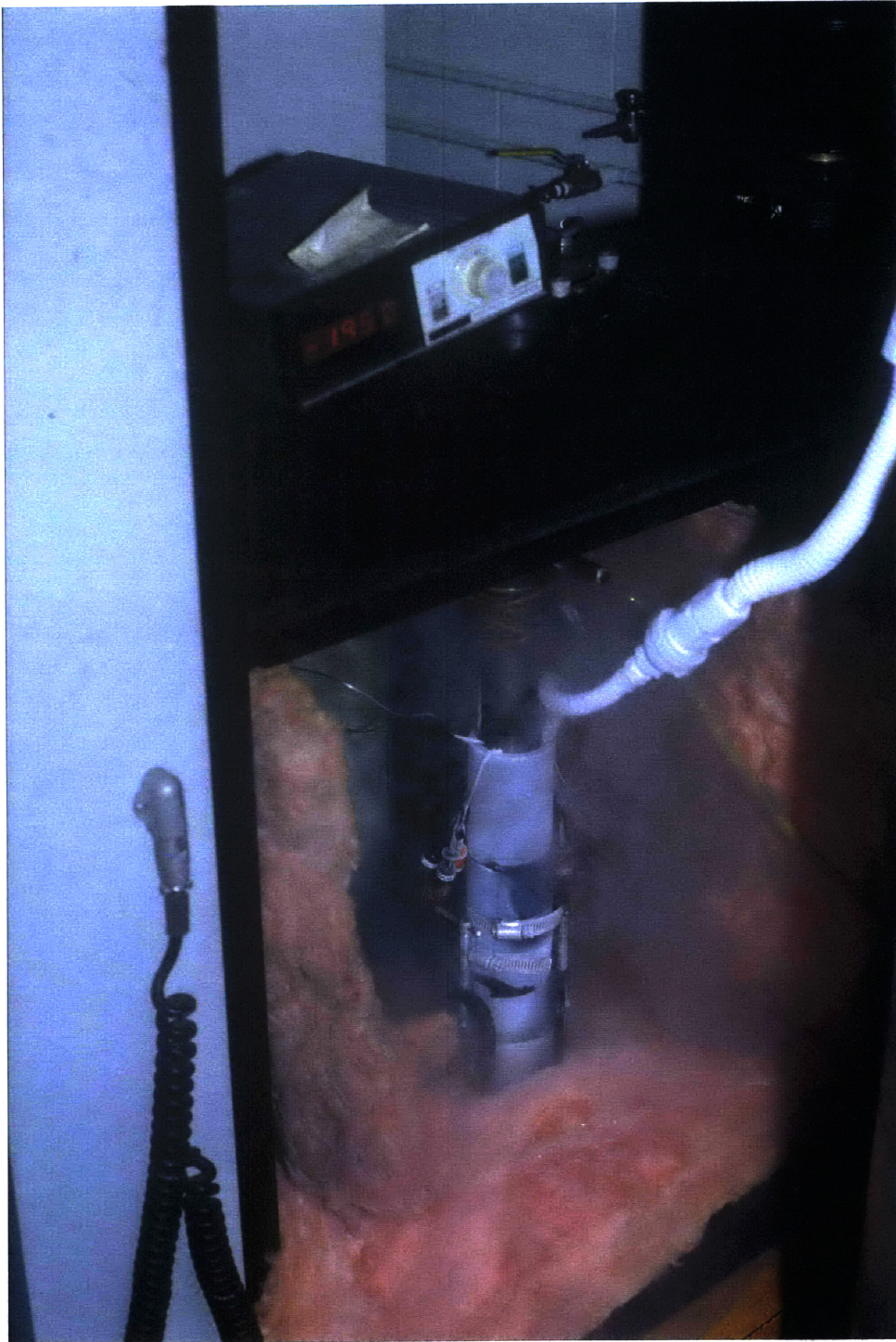
Figure 4-7 - Mechanical test in progress in liquid nitrogen. The temperature reading (-195°C) is from a thermocouple placed near the sample's strain gages.
