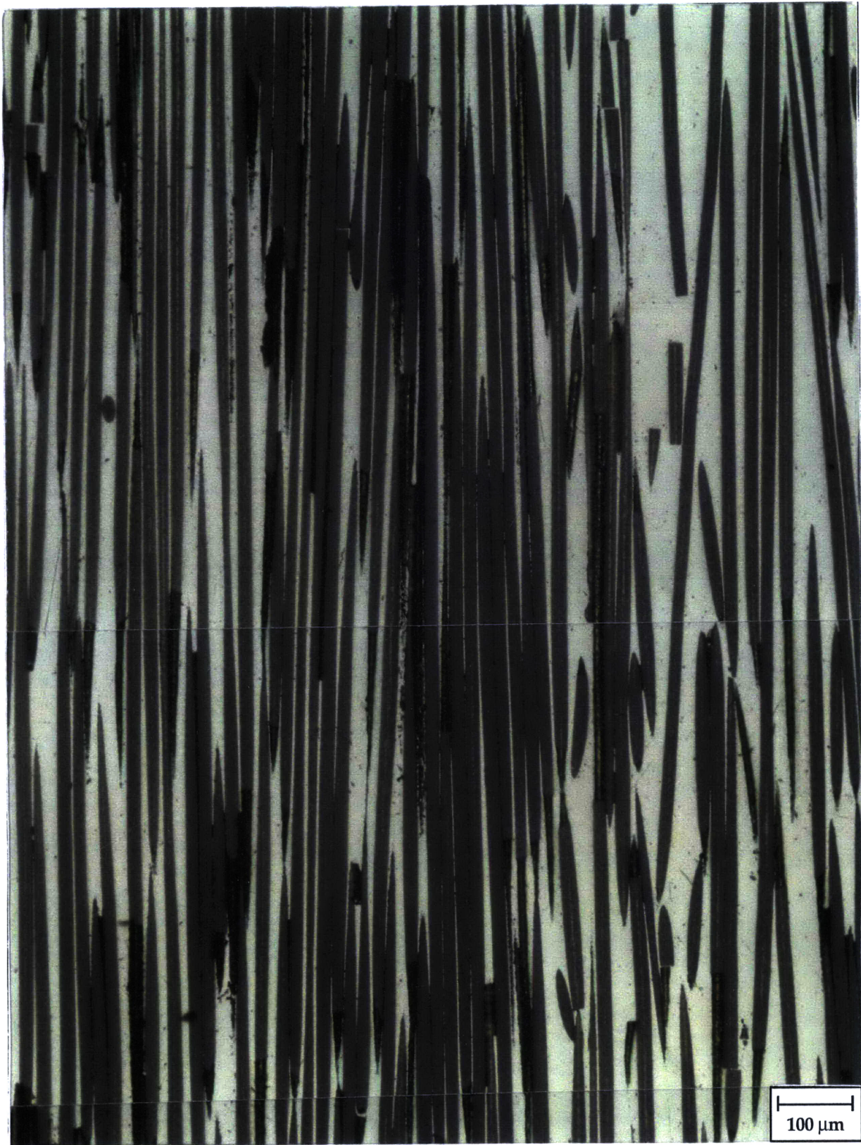
Figure 6-2 - Longitudinal cross-section of Sample 4-2•Cu/FP ( V_f = 60\% ). The area shown is approximately one fifth of that used to estimate the proportion of broken fibers.
