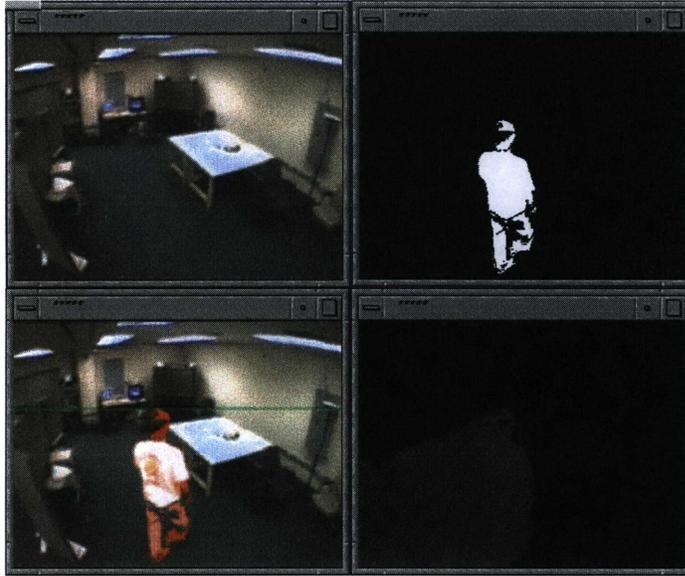
Figure 4-5: *Output of the program run in the example. (upper left) the current background image. (lower left) the current frame. (upper right) the connected component which remained after filtering. (lower right) the current depth map in a very early stage of development. As the depth map is refined, it nears the approximate depth of the scene.*
