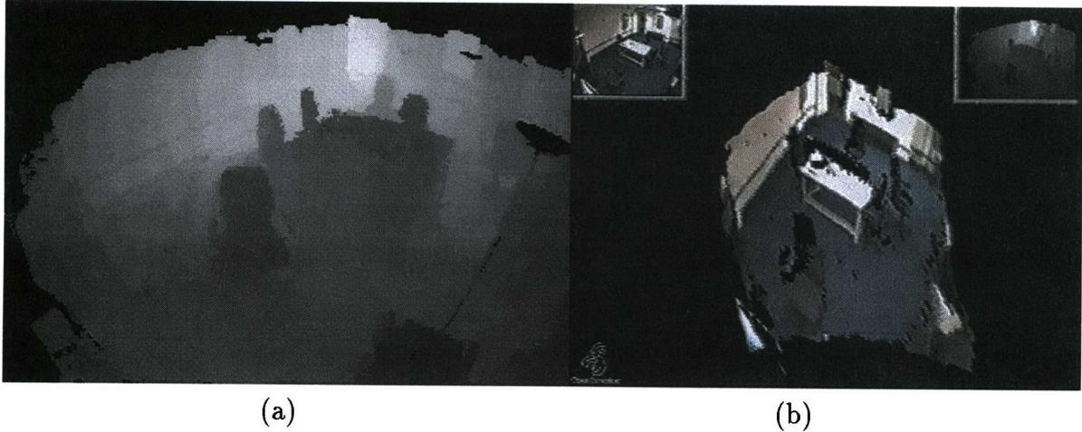
Figure 4-7: (a) The depth map from our example (b) The final output which shows the background used for texture, the depth map used for reprojection, and the resulting model. (center) the resulting model in 3-D.
