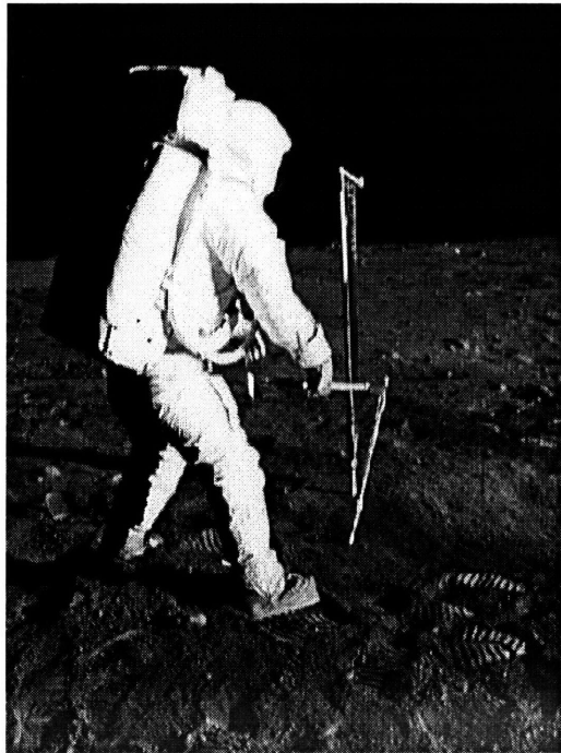
Figure 2-29 – Astronaut “Buzz” Aldrin driving sampling tube with hammer.
