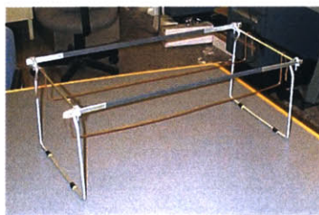
Figure 3.10, Frame Holding the Transilluminator and Gel Tray
