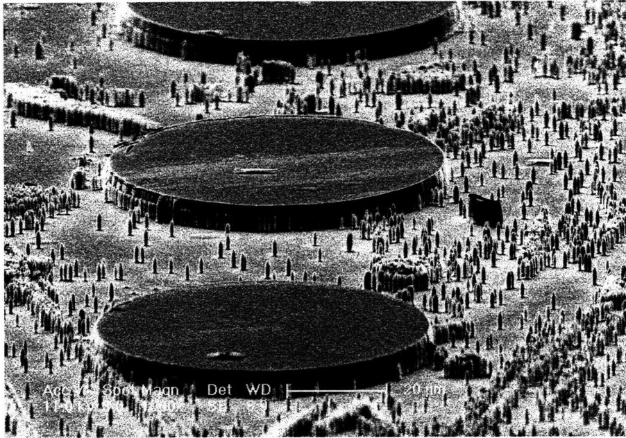
Figure 4-20: Scanning electron micrograph of an array of circular InP-based diodes patterned by reactive ion etching using a methane/hydrogen chemistry.
