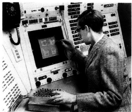
Ivan Sutherland’s Sketchpad console, 1962. Sketchpad is operated with a light pen and a command button box. The four black knobs below the screen control position and scale of the picture.
