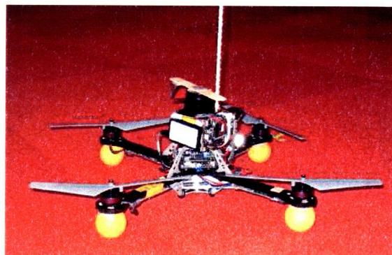
Figure 1-9: A LIDAR enabled quadrotor capable of estimating its position and heading by matching real-time measurements with a map of the room. [57].
