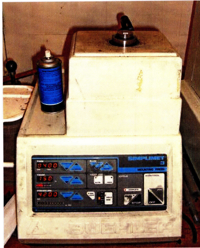
Figure 25: Buehler mounting press used to mount specimens.
