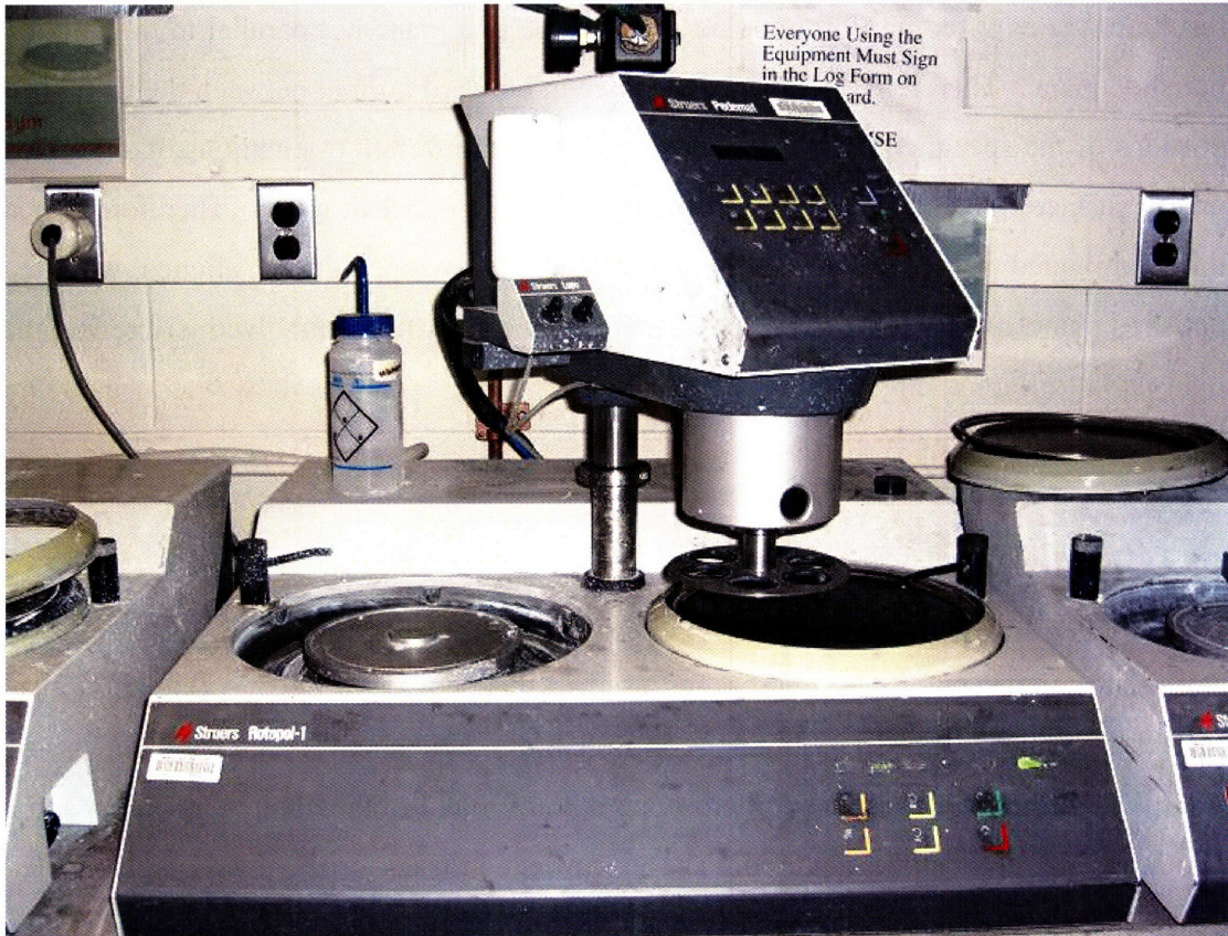
Figure 27: Buehler automatic polishing machine used in grinding and polishing procedures.
