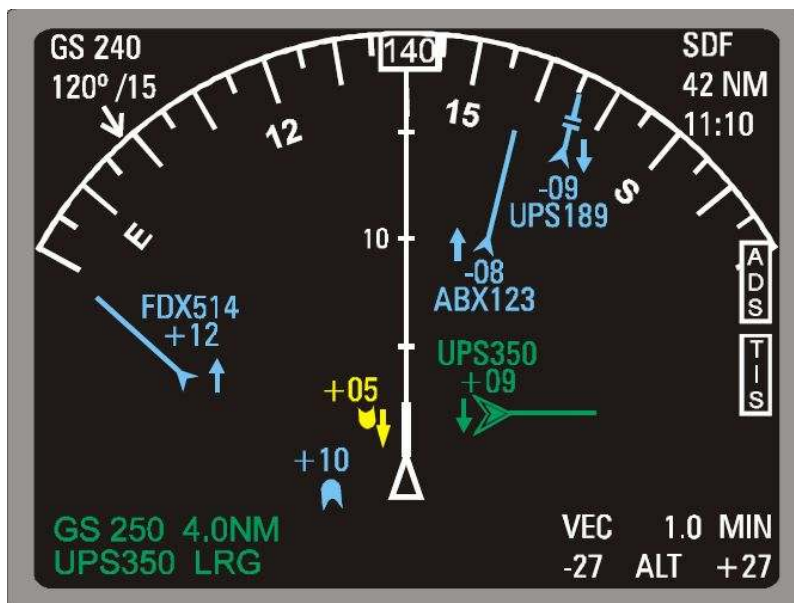
Figure 8: Notional Cockpit Display of Traffic Information (CDTI) depicting traffic identifiers, relative altitudes, and tracks [24]
