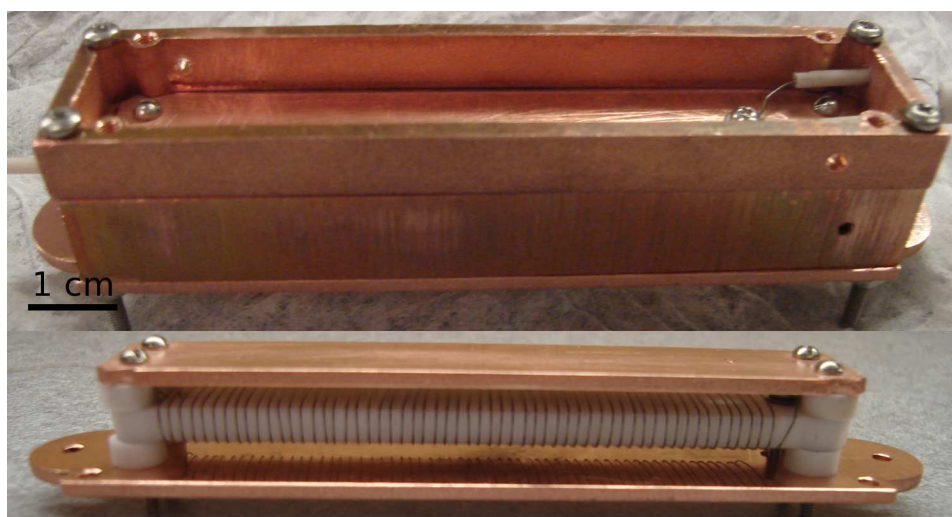
Figure 3-5: (top) Annealing oven designed to heat a sample up to 800 °C in vacuum. (bottom) Heating element, made out of tungsten wire wound on an alumina bar, and contained in the lower part of the oven.
