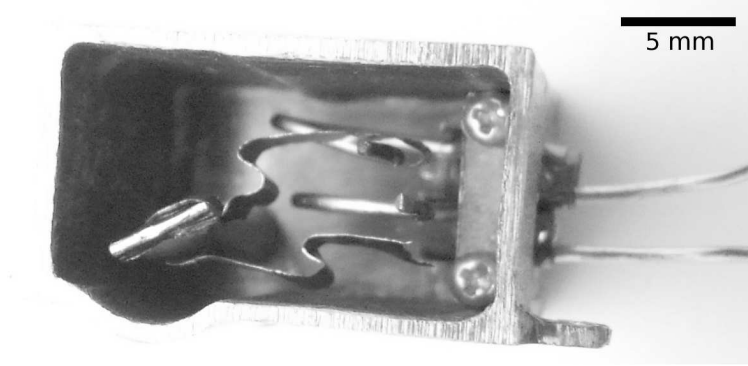
Figure 3-11: Sr oven for the cryogenic environment. Sr metal is confined in a stainless tube, shielded by copper walls from all sides. 0.002" stainless foil is used as a heating element, requiring \approx 5 A to produce neutral Sr vapor.
