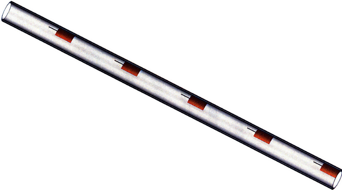
Figure 3-2: Thermocouple placement along confinement tube. Five K-type thermocouples are bonded at equal intervals along the 40 cm length.
