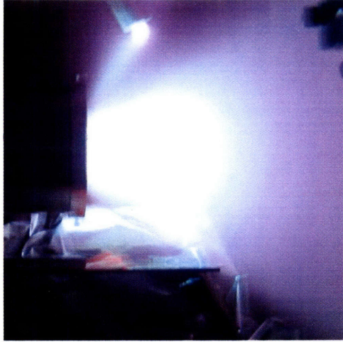
(a) Visible discharge operating in the high anode current mode. Operating with 10 sccm of anode flow and 400 Volts applied to the anode.
