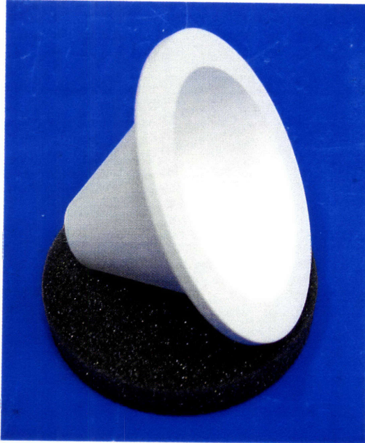
Figure 2-14: The HP grade boron nitride cone used to insulate and protect the DCF channel walls. The cone was manufactured by Saint-Gobain Ceramics[5].
