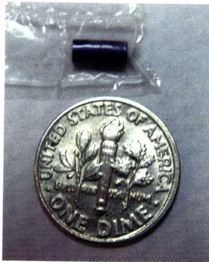
Figure 6-9: One of the LaB_6 inserts used in developing the hollow cathode presented here.
