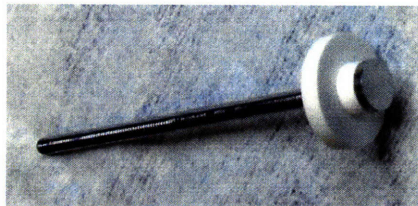
Figure 2-12: Partially assembled stainless steel anode and ceramic spacers.
