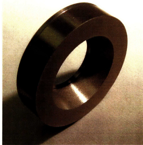
Figure 2-6: One of the SmCo magnets used in the DCF prototype, see appendix A for exact dimensions.
