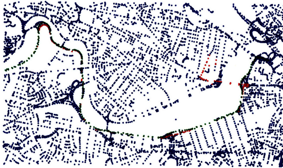
Figure 4-17: Two paths (green overlaid on red) with fewer than 90% of the waypoints in agreement.
