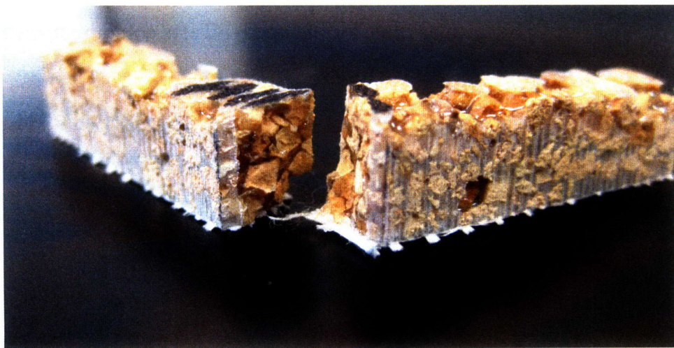
Figure 25: Close-up of cork specimen after undergoing Charpy test
