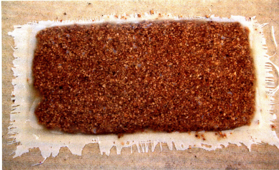
Figure 11: One-sided cork sample, after curing and before machining.
