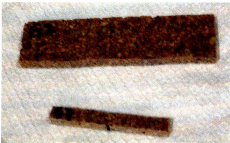
Figure 13: Cork samples machined for the bending test (above) and the Charpy test (below)
