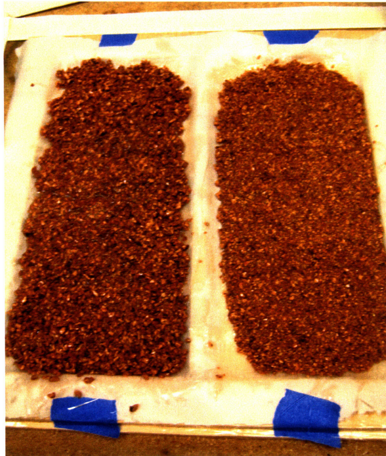
Figure 10: Two one-sided cork samples laid up in half the flat mold.
