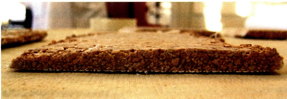
Figure 12: Cross-section of mixed cork sample.
