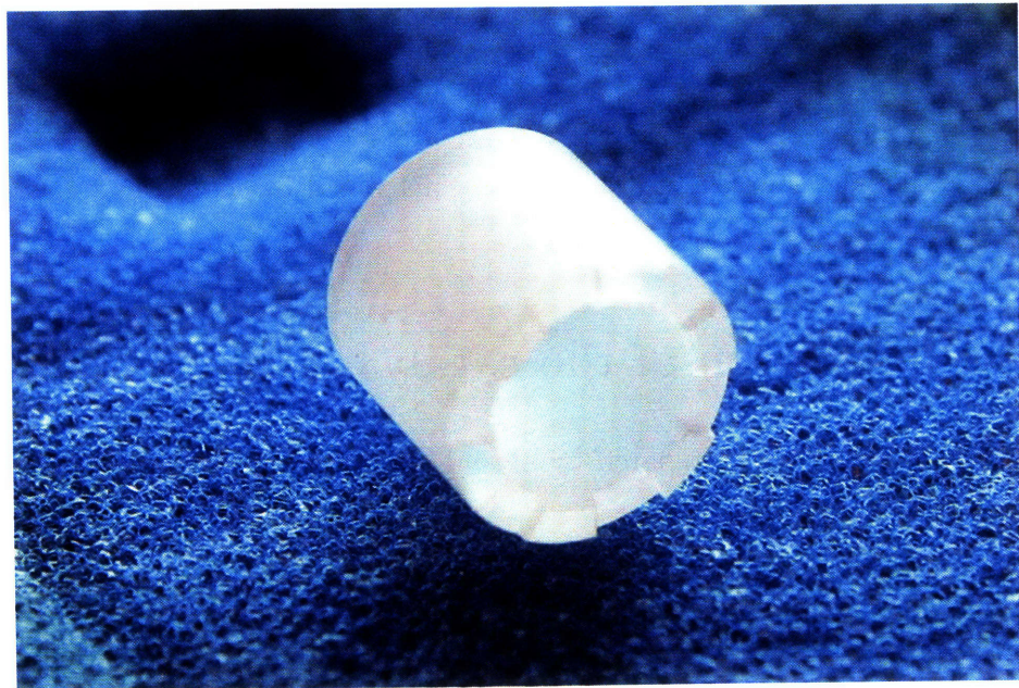
Figure 3-14: Picture of ultrasonically machined exit tube (sapphire)
