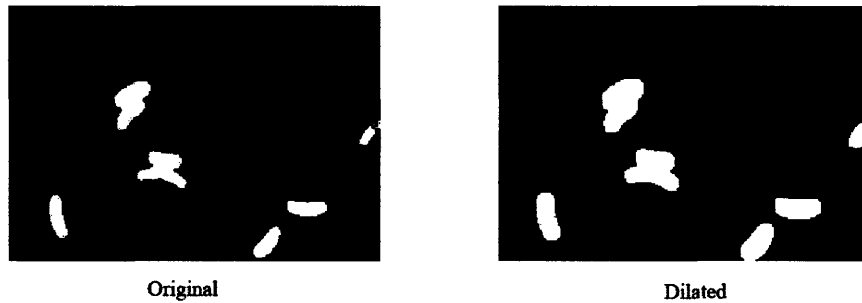
FIG. 5.6: Original binary image and result after dilation with a 5x5 grid.
