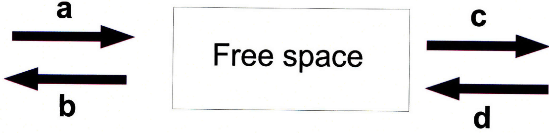
Figure 4-2: The fields entering and exiting a region of free space are shown. Propagation operators are characterized by the propagation distance (and orientation relative to the source polarization, in the case of the GW signal).
