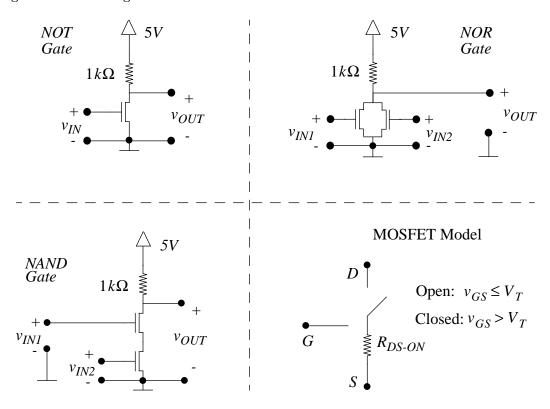
Figure 2: a NOT gate, a NOR gate, a NAND gate, and the switch-resistor MOSFET model.
