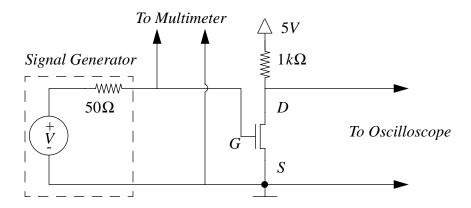
Figure 5: circuit to measure  $V_{\rm T}$ .
