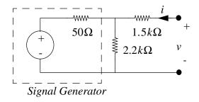
Figure 4: experimental source-resistor network.
