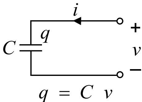
$$\begin{aligned} i &= \frac{dq}{dt} \\ &= \frac{d(Cv)}{dt} \\ &= C \frac{dv}{dt} \end{aligned}$$
