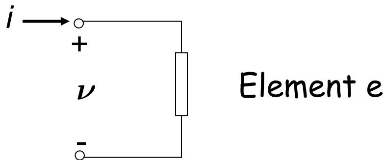
Current is taken to be positive going into the positive voltage terminal
