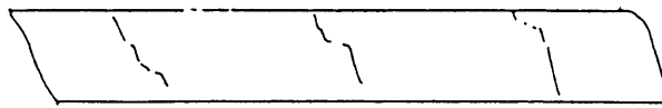
Figure 2.13: Ruptures Observed in Radiograph of Simple Shear Test on Kaolin (sketches of radiographs of threads of lead paste; after Airey, et al., 1985; from DeGroot, 1989).
