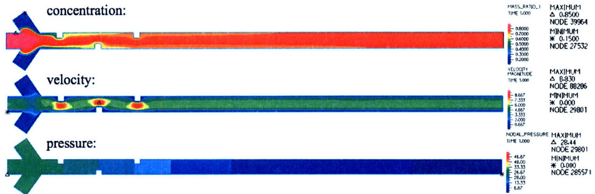
Figure 8d: Simulation results for straight channel mixer with 3 notches
