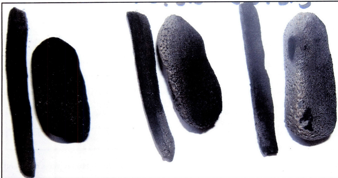
Fig 40 Bodies after having been fired in limited-oxygen environment
