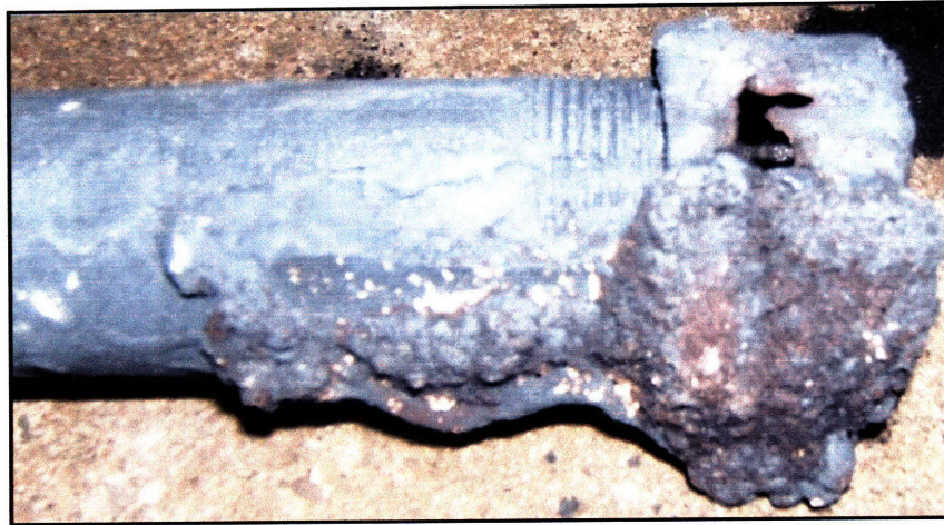
Fig 23 The temperature reached approximately 1250 °C before the kiln was switched off. The black malleable steel end caps melted onto the kiln floor and the nipple.
