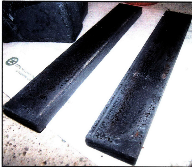
Fig 17 Steel mold bars after exposure to high temperatures in oxidizing kiln environment
