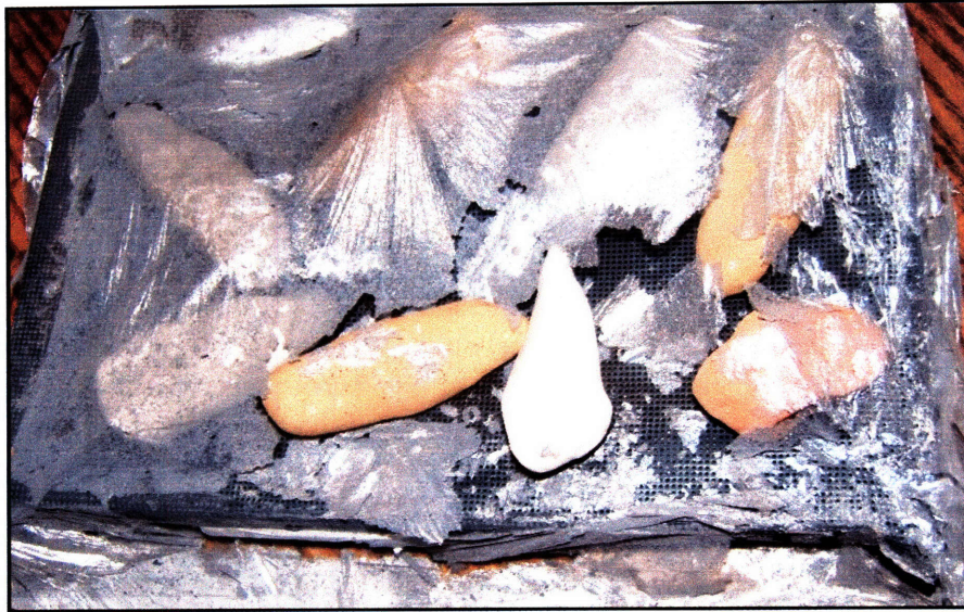
Fig19 Ticonic tool steel foil dissolved after kiln reached 1070 °C
