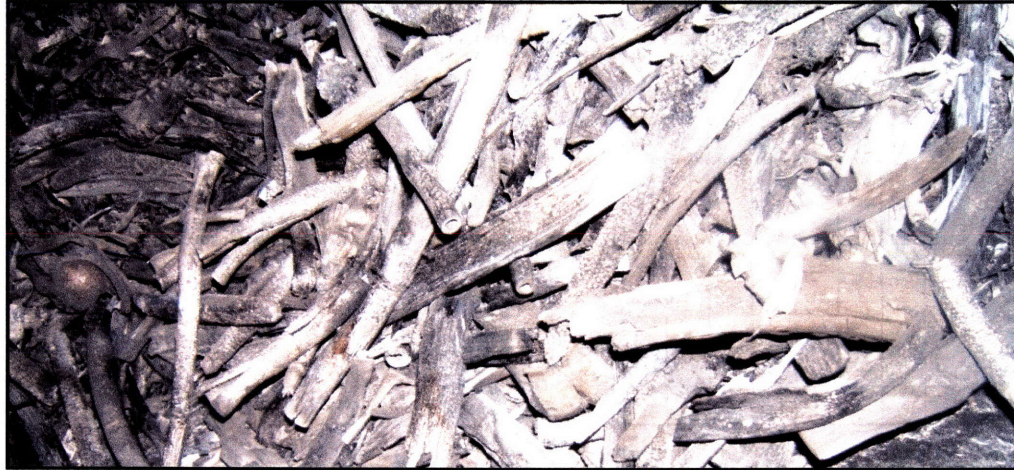
Fig 36 Bamboo that has been carbonized in an oil drum
