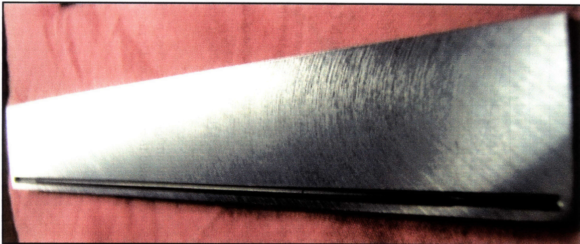
Fig 15 Mild steel bar with pencil lead groove milled along its length
