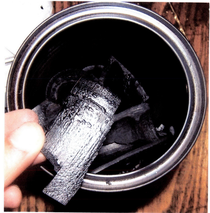
Fig 35 Bamboo charcoal made in a kiln.
