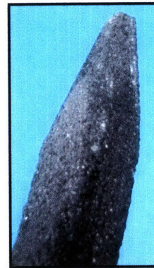
Fig 29 (left) 3:1 clay to charcoal body that has sintered and sharpened; (right) faint marks made by this body scratched the paper
