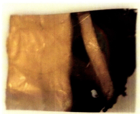
Figure 15: Trial gold-sputtered PVDF membrane with polypyrrole deposition on the left. The gold streak in the middle was due to a plastic piece of the deposition device floating because it was not secured correctly.
