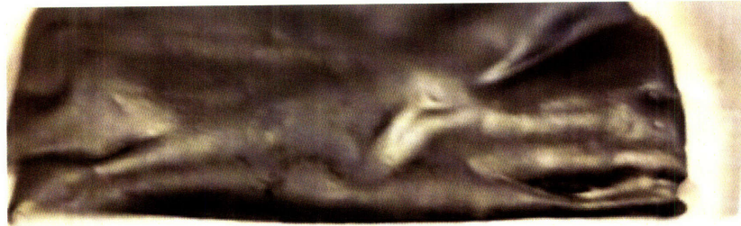
Figure 17: Trilayer deposition using the gold-coated PVDF technique. Polypyrrole is directly deposited onto the gold coating on both sides of the PVDF membrane.
