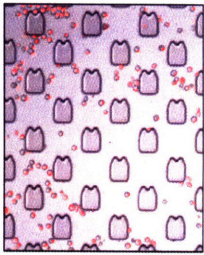
Few cells trapped; poor print resolution
