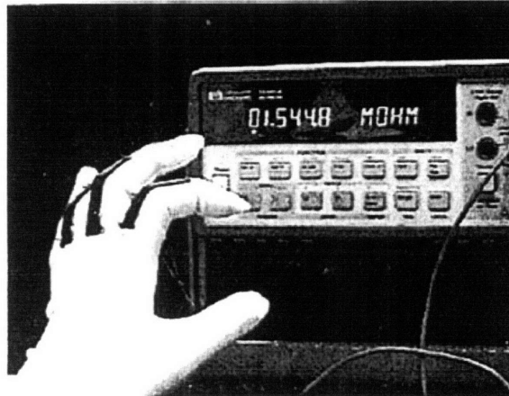
Figure 3-2: Spinks et al. were able to sense the flexure of each finger using the variable resistance of the CP/fabric strain gage mounted on the back of each glove finger (from [37]).
