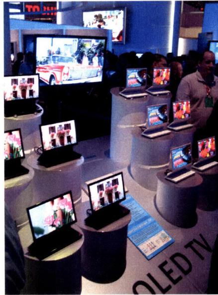
Figure 5-5: . These OLED high definition televisions from Sony® have a contrast ratio of 10^6 : 1 and were first displayed at the 2007 Consumer Electronics Show.
