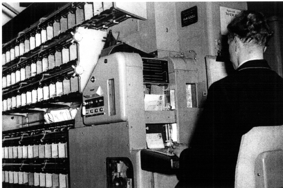
Figure 6.2. APU mechanized letter sorter. From L.A. Reynolds and E.M. Tansey, "The MRC Applied Psychology Unit," Wellcome Witness to Twentieth Century Medicine Vol. 16: 34. http://www.ucl.ac.uk/histmed/PDFS/Publications/Witness/wit16.pdf . Accessed January 23, 2008.
