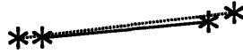
Figure 4-3: An Example of inexact collinearity: The lines are not exactly collinear, but we should probably detect them as such.
