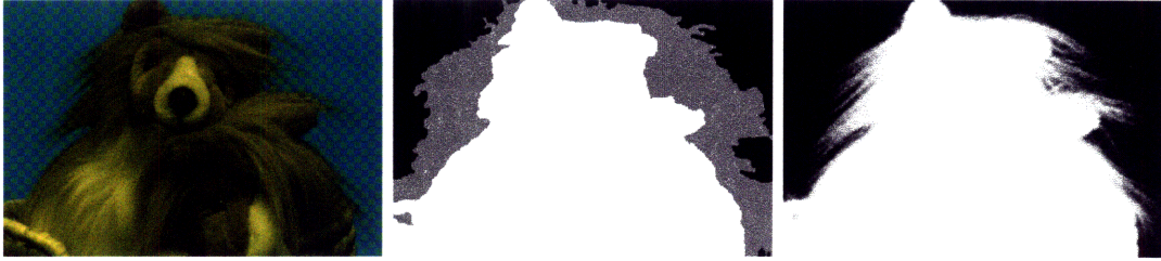
Figure 1-2: Example of a trimap. From left to right: Original Image, Trimap, Alpha Matte generated using Bayesian Matting [9]. In the trimap, black represents background, white foreground, and gray unknown.
