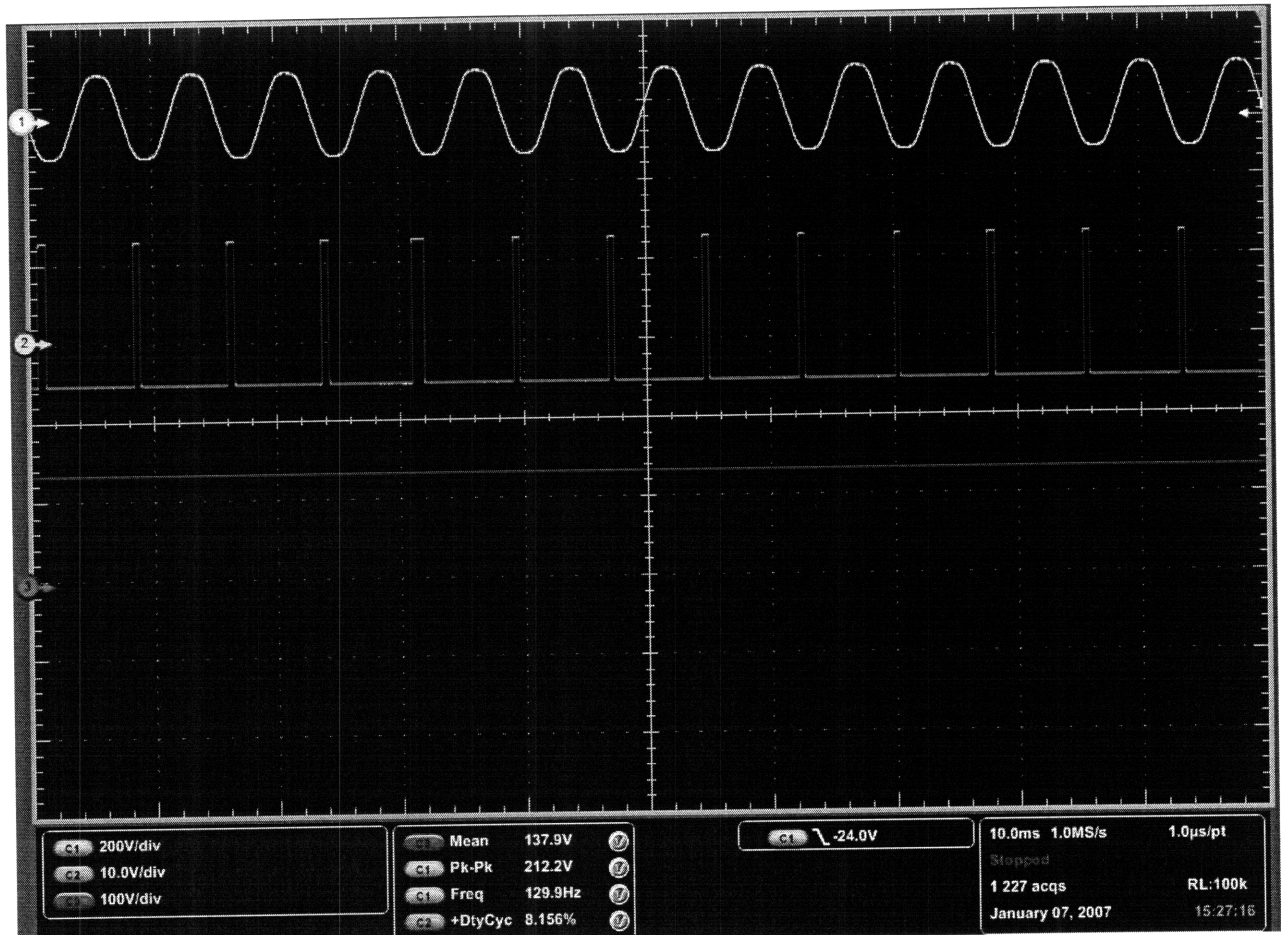
Figure 6-4: Gate-drive duty cycle (trace 2) approaching zero since the load was increased above the reference. Trace one is the line-to-neutral voltage, trace two is the IGBT gate-drive signal, and trace three is the load voltage.
