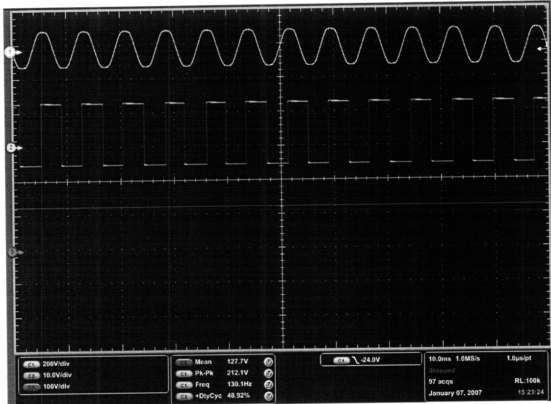
Figure 6-2: High duty cycle gate-drive (trace 2) because load is held below reference. Trace one is the line-to-neutral voltage, trace two is the IGBT gate-drive signal, and trace three is the load voltage.
