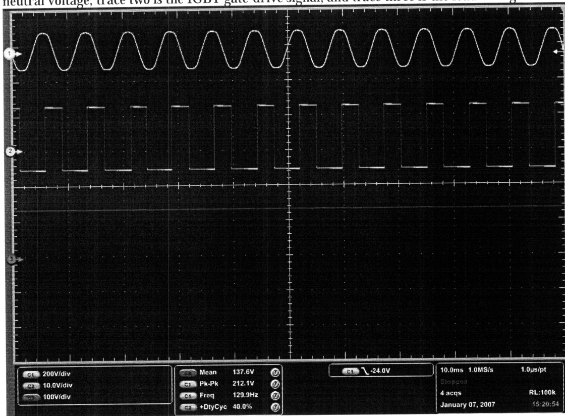
Figure 6-3: Gate-drive duty cycle (trace 2) is decreasing since the load voltage was increased. Trace one is the line-to-neutral voltage, trace two is the IGBT gate-drive signal, and trace three is the load voltage.
