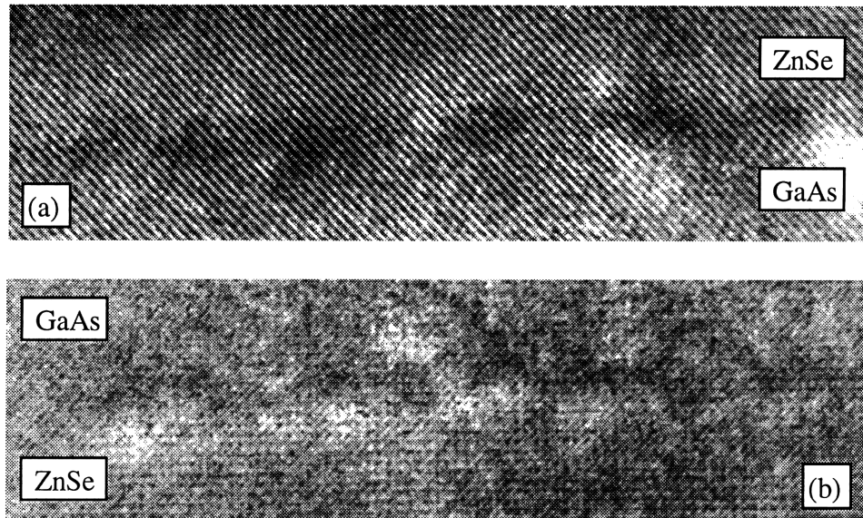
Figure 8-18. HREM [001] lattice image of the ZnSe-on-GaAs heterointerface and the GaAs-on-ZnSe heterointerface for the sample shown in Figure 8-17 (a). Thickness variation across the sample results in the upper interface showing fringes as opposed to the actual lattice.
